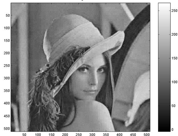
Fig07 Denoised Image using the Wiener Filter in the Wavelet Domain with known noise variance
