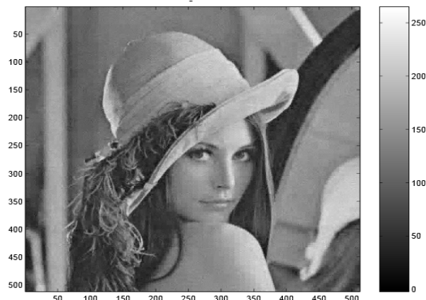
Fig06 Denoised Image using the Wiener Filter in the Wavelet Domain. The noise variance was estimated using the MAD method.
