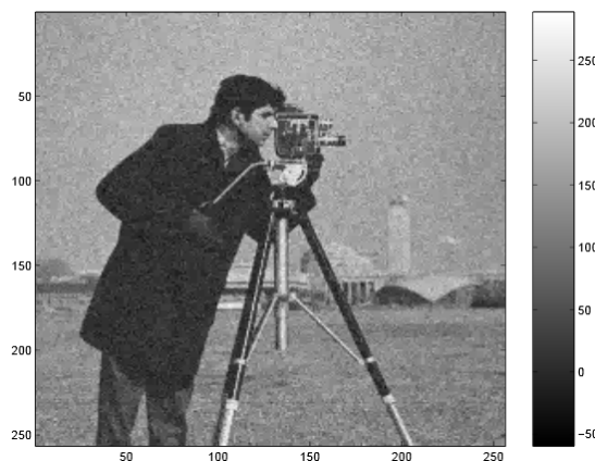
Fig09 Denoised image obtained after thresholding the noisy wavelet coefficient with the Hard Threshold.
