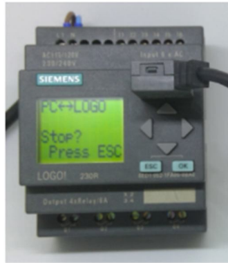
Figure 3: LOGO! PLC Screen Display (Sander van de Velde, 2019).
