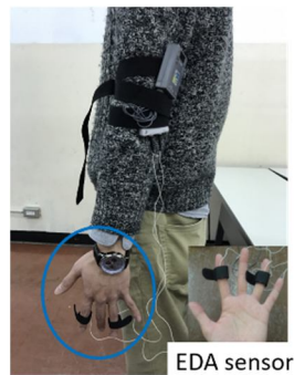
Figure 9: Subject wearing the electrodes for measuring the EDA.
