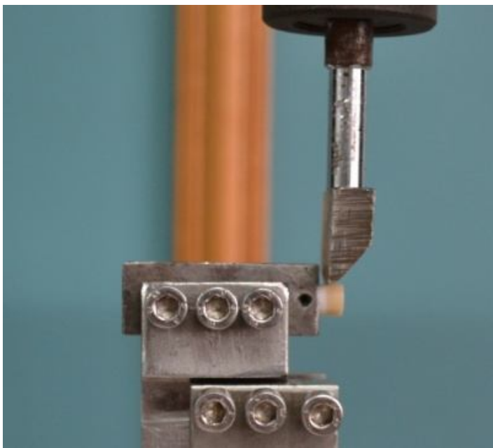
Figure 2: shear bond strength test on specimens
