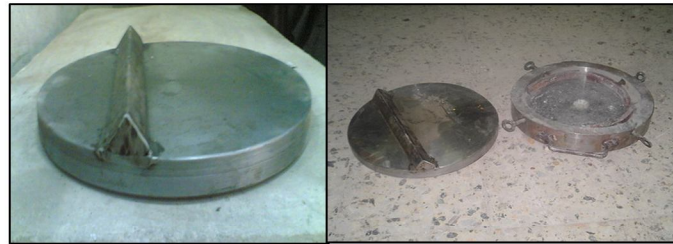
Fig. 5 The eccentric loading mechanism
