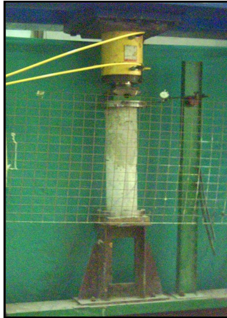
Fig. 7 Typical setup for repair column under load
