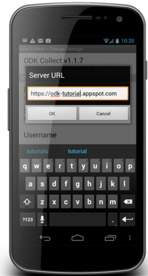
Fig 3.b The Settings Menu: URL Configuration .On the settings Menu configure the URL of ODK Collect to point to the URL of where the ODK Aggregate is deployed in order for retrieval of blank forms and submission of finalized forms to take place
